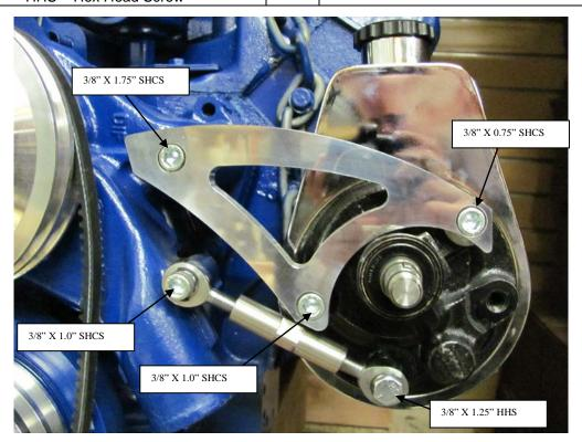
Step 1: Remove old power steering bracket.
