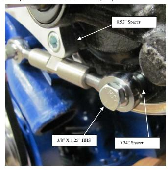
Step 5: Attach adjusting Rod to power steering pump using 3/8 X 1.0" SHCS with 0.34" Steel Spacer between pump and adjusting rod.
